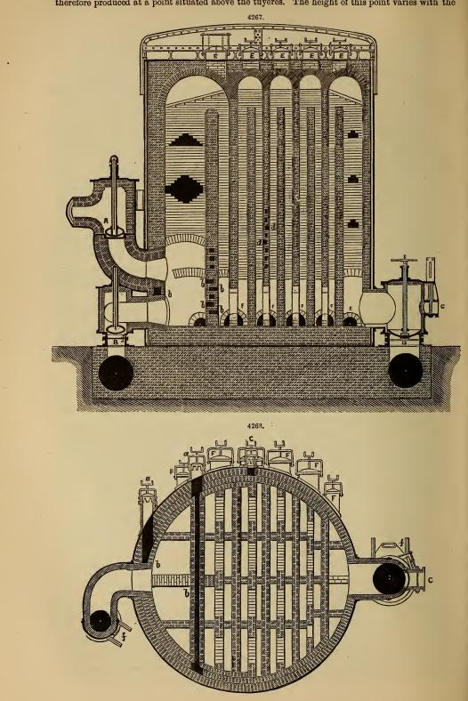
of the fuel, must first be diffused through the fuel before it can burn, and the greatest heat is therefore produced at a point situated above the tuyeres. The height of this point varies with the respective quantities of fuel and of blast that are introduced; and when sufficient fuel is supplied, the point of greatest heat will be situated at the level, where all the oxygen in the blast has
